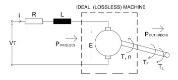
Consider the motor supplied by a terminal voltage (V) supplying a current (I) so that the motor develops a steady torque (T) at speed (n). All motor losses (iron loss, copper loss, windage, friction, brush voltage drop) are modelled by a single resistance R whose power dissipation at current I equates to the motor input losses. Therefore the electrical power into the ideal motor (devoid of its losses), Pin (elec) = E I (watts).
