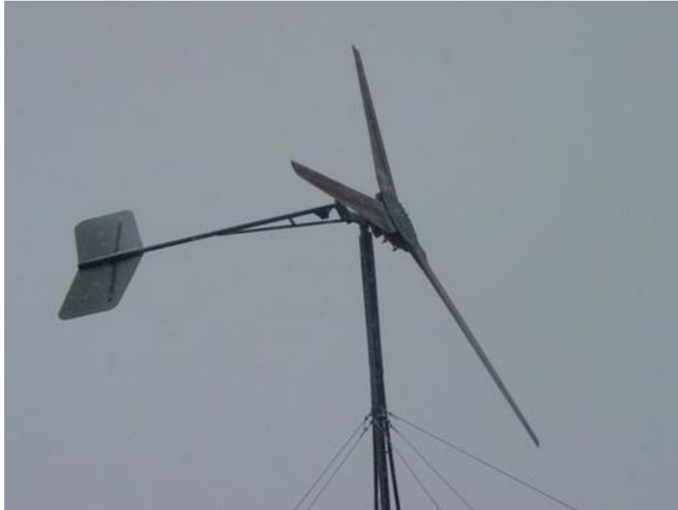
A Successful 17' Wind Turbine Design by Dan Bartmann ( www.otherpower.com )
